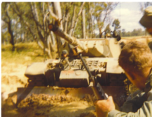
20 Armoured exercise 'Rock Wallaby'. Time out taken to observe Leopard dozer tank and tank bridge layer enabling M-113 APC crossing with dismounted infantry support
